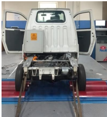
Fig. 5. Performance test on dynamometer
