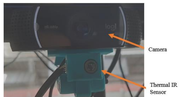
Fig. 6. Thermal sensor installation
