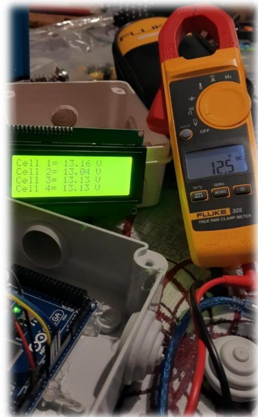
Fig.8. Comparison of voltage measurement by using sensors arrangements and Fluke voltage measurements.
