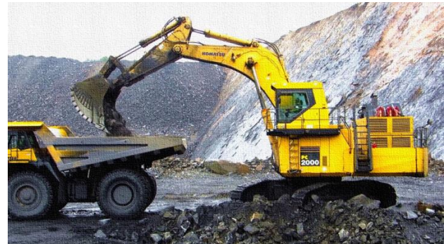
Fig. 1. Hydraulic excavator 200 ton
