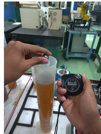
Fig. 1. The process of measuring viscosity using the manual method
