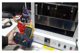
Fig. 5. The comparison of temperature measurement of DHT22 sensor and krisbow digital thermometer
