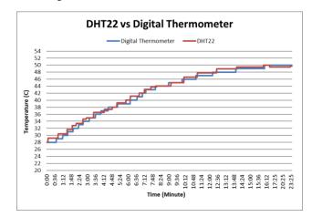
Fig. 6. The comparison of reading temperature result between DHT22 sensor and krisbow digital thermometer
