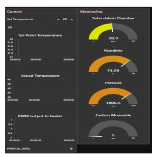
Fig. 7. Dashboard of ETC monitoring system in webserver
