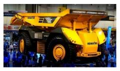
Fig. 2. Komatsu autonomous haul vehicle
