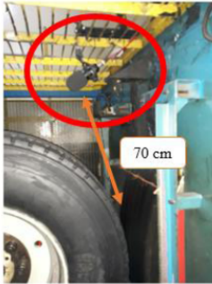
Fig. 4. BM800 in TBR Drum Test Machine.
