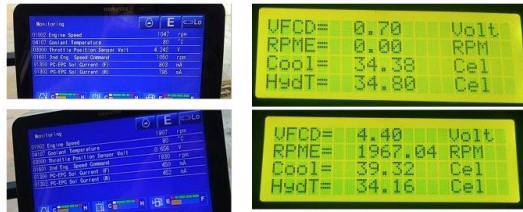
Fig. 10. Comparison of monitoring panel from the actual monitor panel and the simulator.
