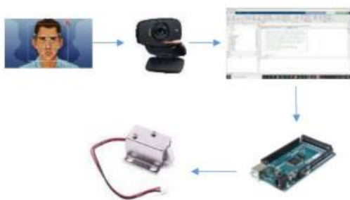
Fig 5. System flow process
