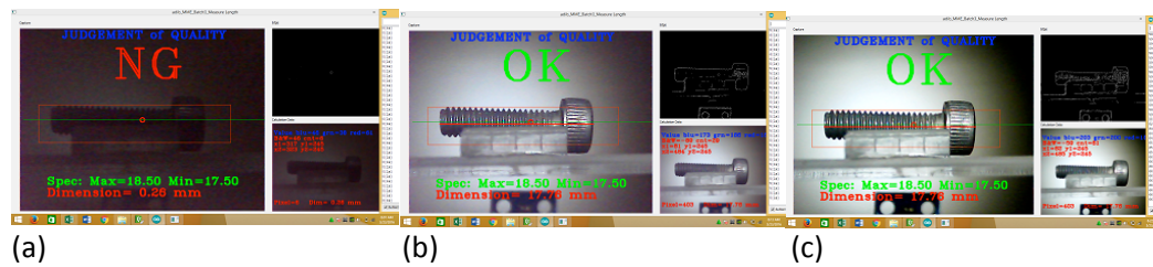
Figure 3. Light intensity 4 Lx (a), Light intensity 10 Lx (b), Light intensity 59 Lx (c).
