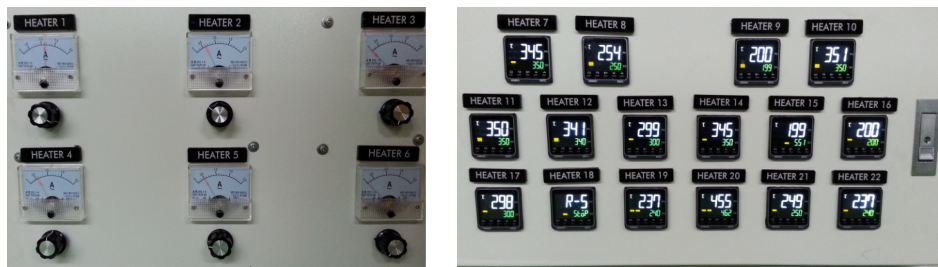
Fig. 8 Non-feedback and feedback control for ceramic heaters in PET vacuum forming application.
