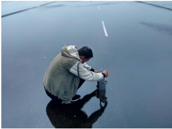
Figure 8. The water depth measurements at Proving Ground Test Track Karawang.
