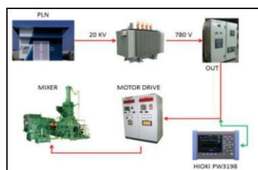
Figure 2 Schematic Measurement output transformer.
