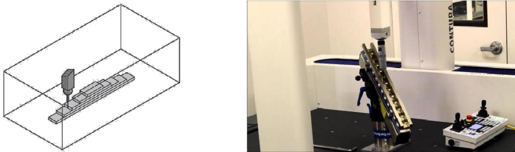
Figure 4.1. Measurement line in calibration procedure on five calibrated lengths reference block along a CMM axis.
